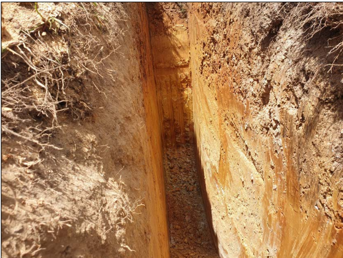
Photograph 12: Phyllite bedrock encountered within test pit advanced for geotechnical investigation (18 November 2020).
