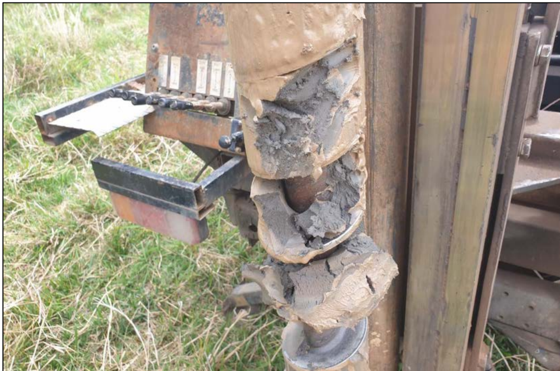
Photograph 8: Grey natural clay material (alluvial soils) encountered beneath detected groundwater (3.0mBGL), within borehole 'BH112' during ASS investigation (17 November 2020).
