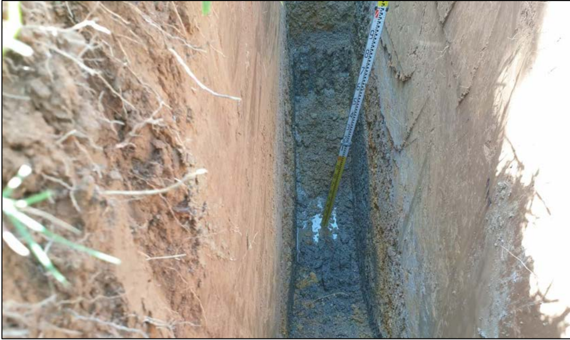
Photograph 11: Groundwater encountered within test pit advanced for geotechnical investigation (18 November 2020).
